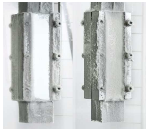
Figure 6 Scaling test in saturated CaSO 4 solution after 24 h Left: CVD-coated shiny aluminum plate without deposits Right: crystal growth on the entire surface of the uncoated reference piece
