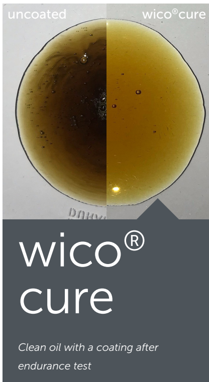
Aging test with mineral oil (SAE-W30) in copper-brazed heat exchangers after 2,000 hours at 120 °C (393 K).
